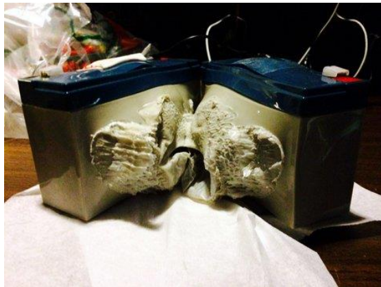
Example of batteries overheated during charging
