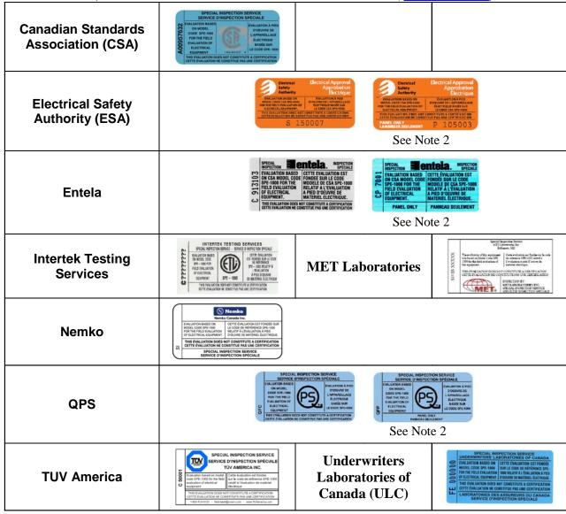
**Note** -"PANEL ONLY" label identifies that the panel has been evaluated to the SPE-1000. It does not cover equipment that is added or connected to the panel.
