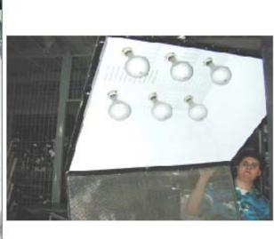
Specifications: Fabricated from a metallic non flammable enclosure. This fixture is used as an overhead softlight. Often this fixture is found with a black fabric drape hung around the bottom so as to direct light straight down.
